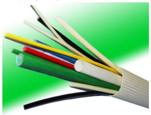
Acrylic fiberglass sleeving is made of non-alkli fiberglass with acrylic resin coating, it has reliable heat resistance, widely used as wiring insulation for motors, electrical appliance, etc.
